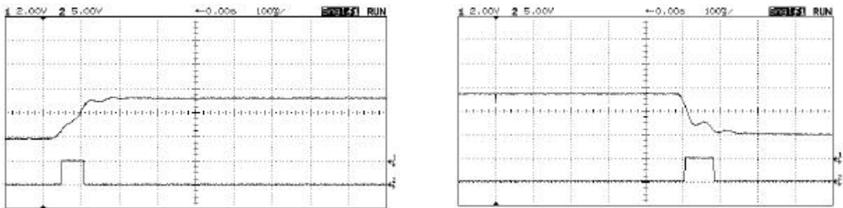
Fig. 3 Experiment results upper curve - torque changes taken from OPM , lower - position signal from HP HEDS5500 , left second coil turned on, right - off (0.5 A constant current power supplying, half step mode, flywheel - 1300 gcm 2 )
