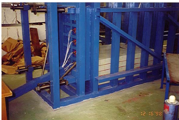
Figure 2: Experimental stand with arbitrarily moved front wall (blue). The wall is the plane inside the structure on the left. Four red bi-component sensors can be seen placed in the front retaining wall. The first above is not in place. The sample is not finished.
