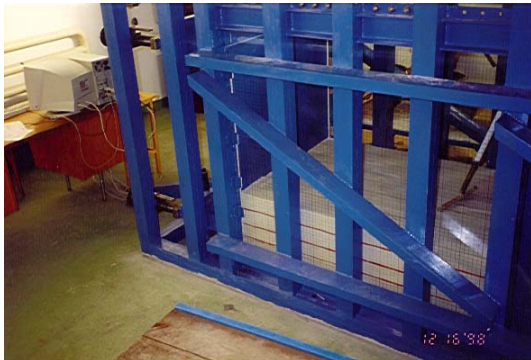
Figure 1: Experimental stand inside as seen through transparent lateral sides. The retaining wall is the blue plane inside the structure on the left. Five bi-component sensors placed in the retaining wall cannot be seen behind the steel column. The sample is not finished.
