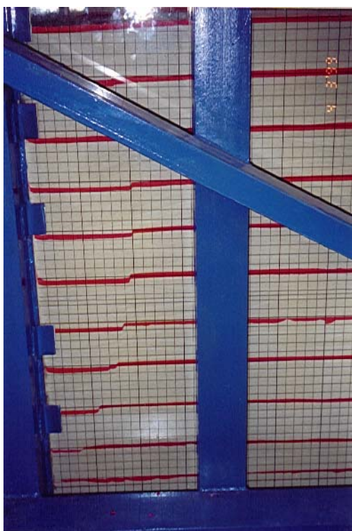
Figure 3: Curved slip surface in the mass after active front wall rotation (left) about the top ( out of mass ). The toe movement was of 8.75 mm; the mesh size 20/20 mm.
