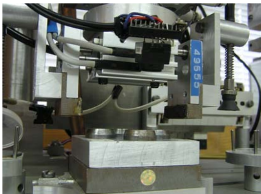
Figure 11. Camera module on the handling arm
