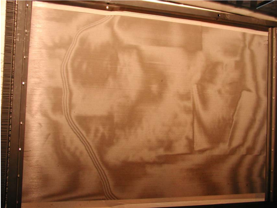
Figure 3 Shadow moiré fringes depicting the state of slip surface in the final loading stage of experiment E3.
