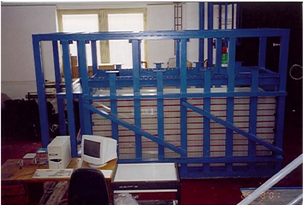
Figure 1 The state of the mass and the first glass plate before the wall movement (rotation about the top - the moved wall is left) on 6th Sept. 2002.
