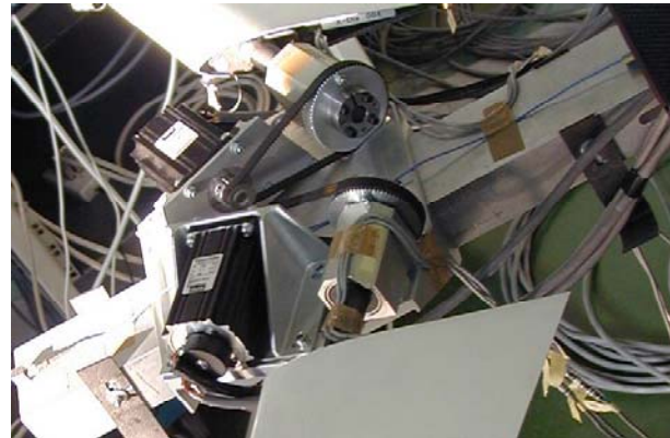
Fig. 5 Detail of the foreplane drive system
