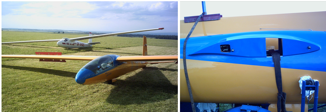
Figure 9: VSB-62 and VT-16 sailplanes, wing root of VSB-62 (Eppler STF 863-615), photo ©Jan Rensa jr.
