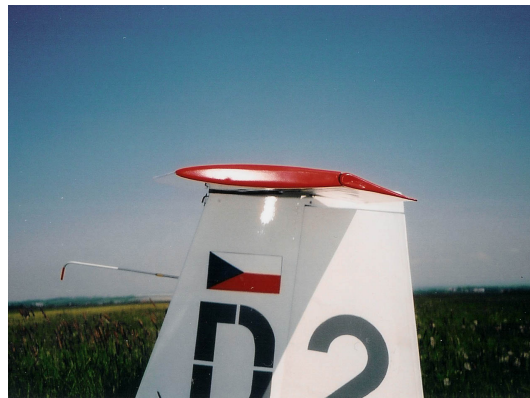
Figure 12: Horizontal stabilizer of VSO-10C OK-0530 sailplane, elevator deflection \gamma = +16^\circ , photo ©Aeroklub Polička
