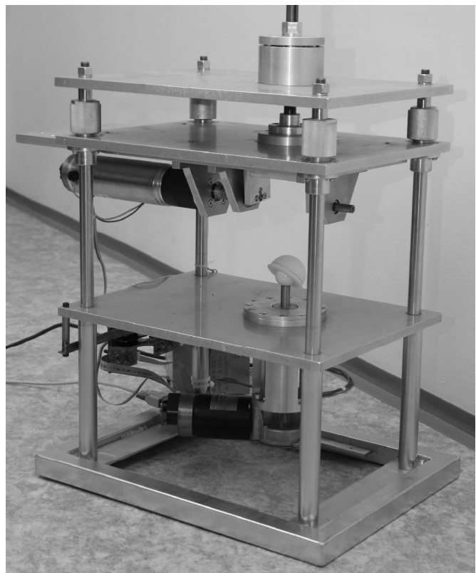
Fig. 2: Experimental device for testing of the wear of polyethylene cups
