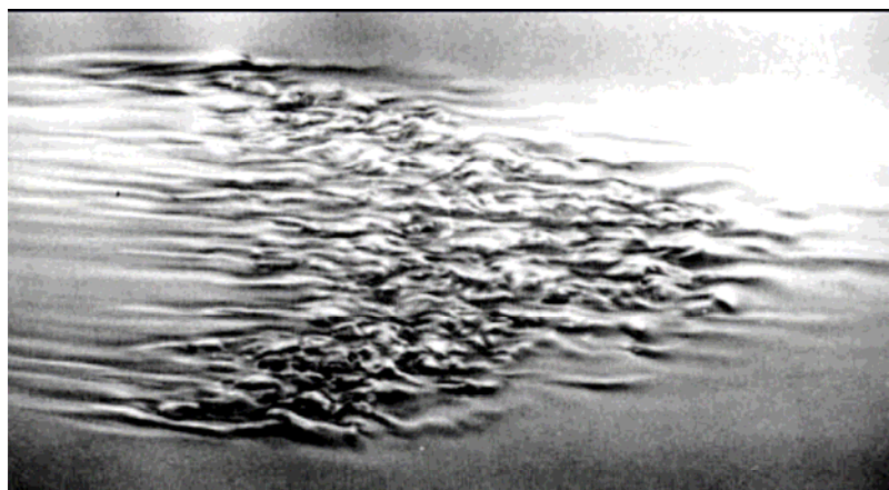
Figure 2. Spot flow visualisation showing the sublayer streaks (Cantwell et al., 1978; copied from Krishnan & Sandham, 2006).
