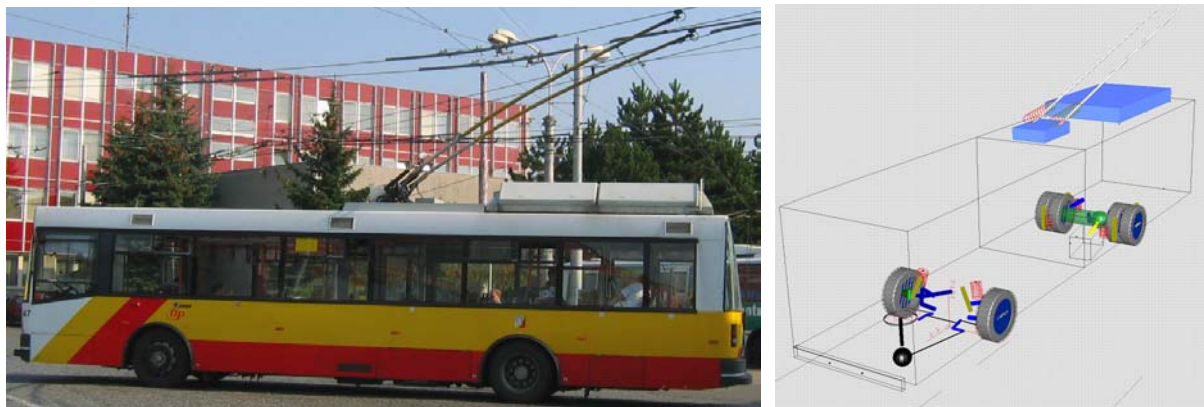
Fig.1 The ŠKODA 21 Tr low-floor trolleybus – the real vehicle and the multibody model visualization in SIMPACK simulation tool.
