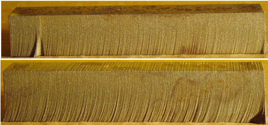
Fig. 2. Typical walls of samples cut by abrasive water jet – the quality is decreasing with the increasing depth (thickness) of cut-through material.
