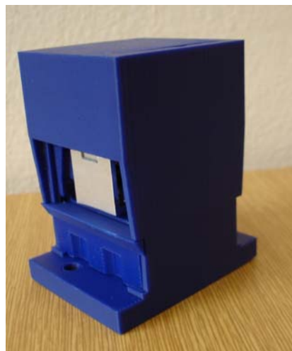
b) Plastic housing of generator and electronics
