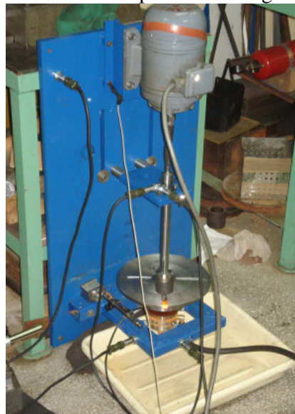
Fig. 5. Stand for determination of bearings parameters
