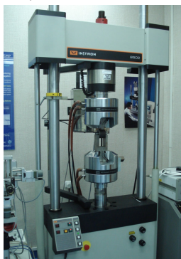
Fig. 10. Testing stiffness in static and dynamic ways on INSTRON device
