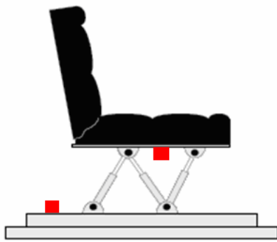
(a) Planar electro-hydraulic AVCS (Klooster, 2003)
