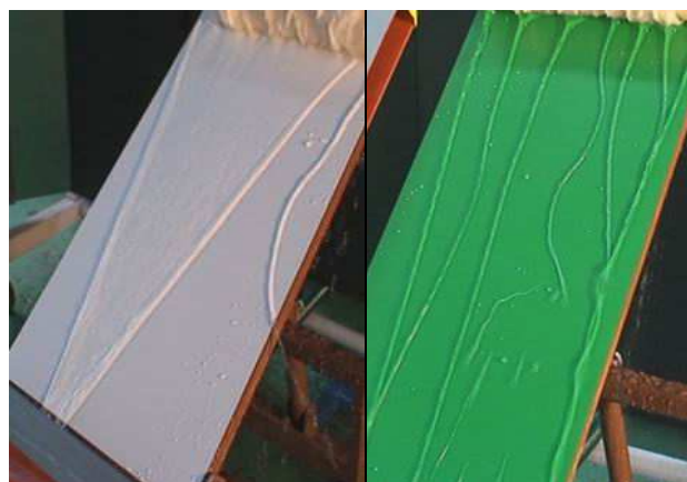
Fig. 3 The liquid layer running down on the inclined plane
