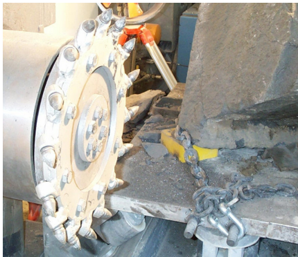
Figure 1 Typical Example of Mechanical Interaction between Bits and Hard Rock (Ore Disintegration Process).
