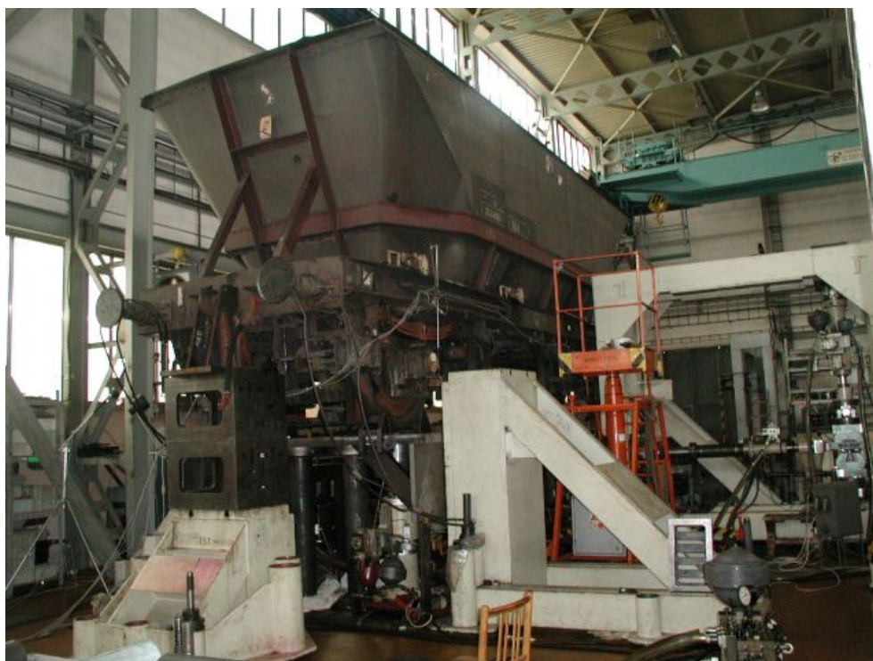
Fig. 1 The MGR Coal Hopper HAA wagon on the test stand.
