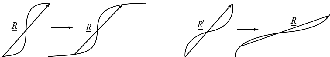
Fig. 1 Influence of the primitive path of a molecule on its final end-to-end vector \underline{R}
