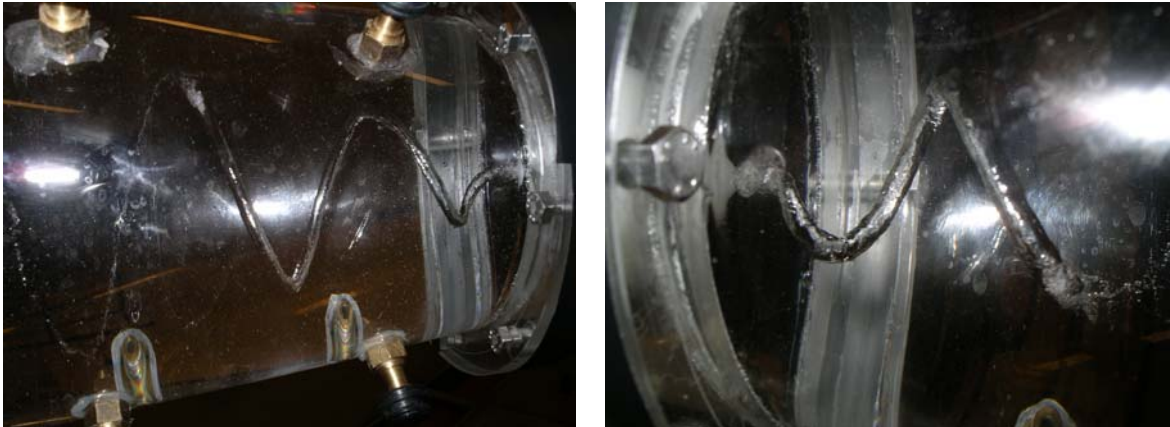
Fig. 1 Cavitating vortex rope (experimental visualization, Rudolf(2009))
