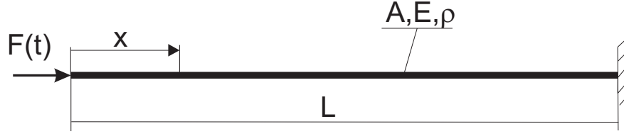
Figure 1: One-dimensional bar under force loading.
