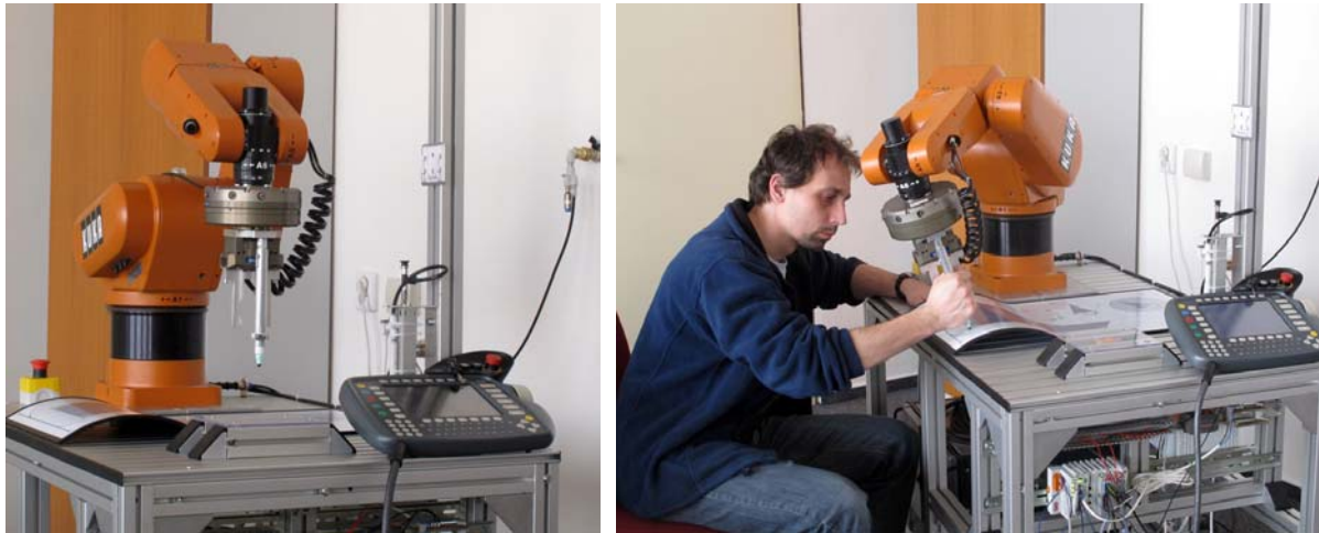
Figure 6 Experimental set-up of FTC robot control for “programming-by-demonstration”
