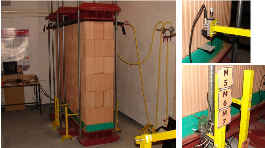
Fig. 6: Stressing frame and detail of mechanical sensors.
