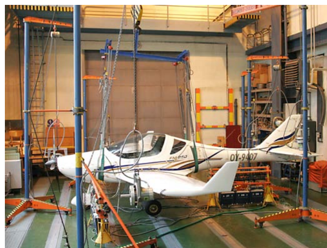
Fig. 2: GVT test arrangement (source: VZLU)
