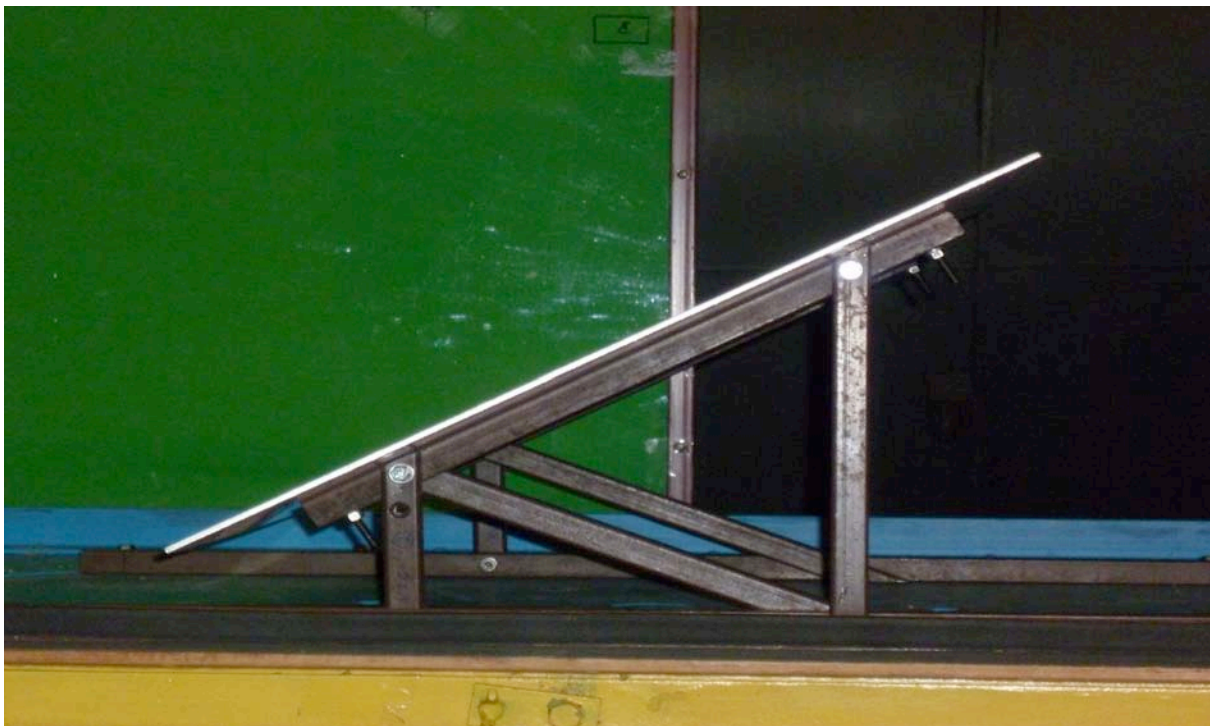
Fig. 1. Side view of the skew plate studied in aerodynamic tunnel
