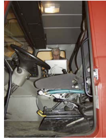
Figure 2. Active seat with a dummy in laboratory and in the truck
