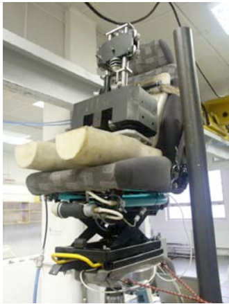
Figure 2. Active seat with a dummy in laboratory and in the truck
