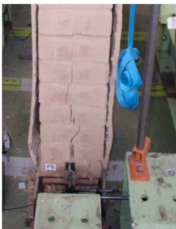
Fig. 15: Vertical crack in the wall thickness
