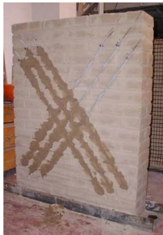
Fig. 3: Adobe brick wall with a steel wire ropes (ABW_2)
