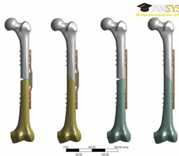
Fig. 1: Complete four virtual models of fractured femur diaphyses with internal osteosyntheses
