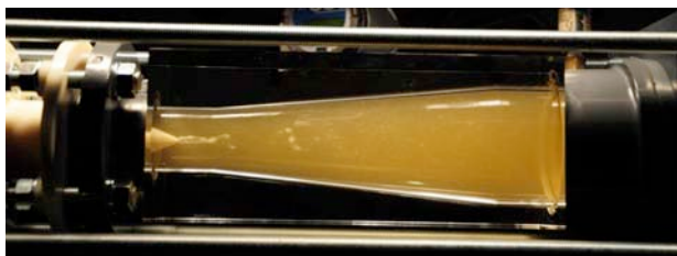
Fig.3: Cavitating vortex rope (experiment)
