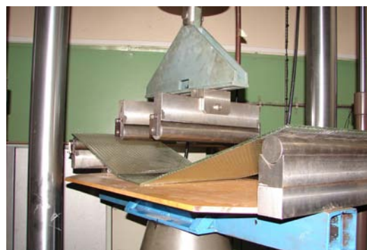
Fig. 2: Four point bending test on wire glass
