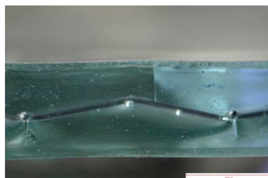
Fig.5: Notches caused by the cutting
