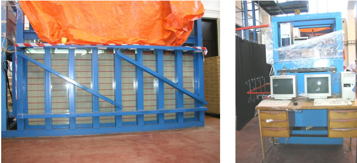
Fig. 1. Experimental equipment with transparent glass sides before experiment E6/02 with non-cohesive sandy sample into:
