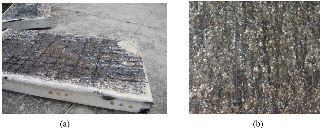
Fig. 3: Specimens after an experiment: (a) FAC2 mixture, (b) FiFAC2 mixture (PP fibres included)
