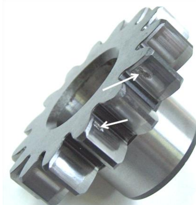
Fig. 1: Pitting damage of real gear.
