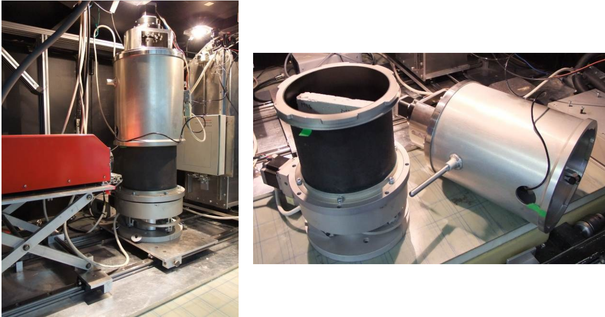
Figure 2: Radiographic setup with loading device left. Disassembled chamber with the specimen right.
