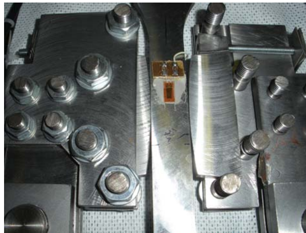
Fig. 4: Detail of the fretting pad installation in the experimental equipment – the original configuration without chamfers.
