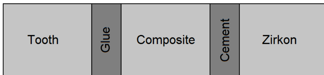
Fig 4. Schematic presentation of multilayer laminated connections
