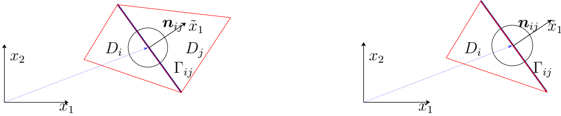
Figure 1: Coordinate transformation for the inner and boundary edges in 2D (inner edge left).
