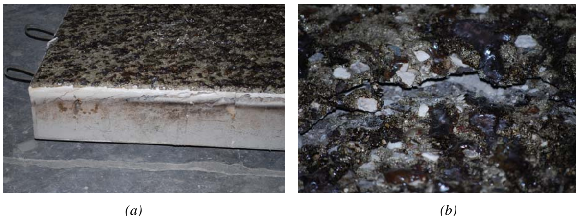
Fig. 3: Specimens after an experiment: (a) FiFAC3 mixture, (b) FAC3 mixture - detail
