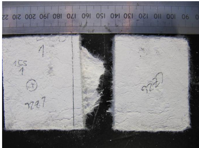
Fig. 4: Shear failure of the specimen.
