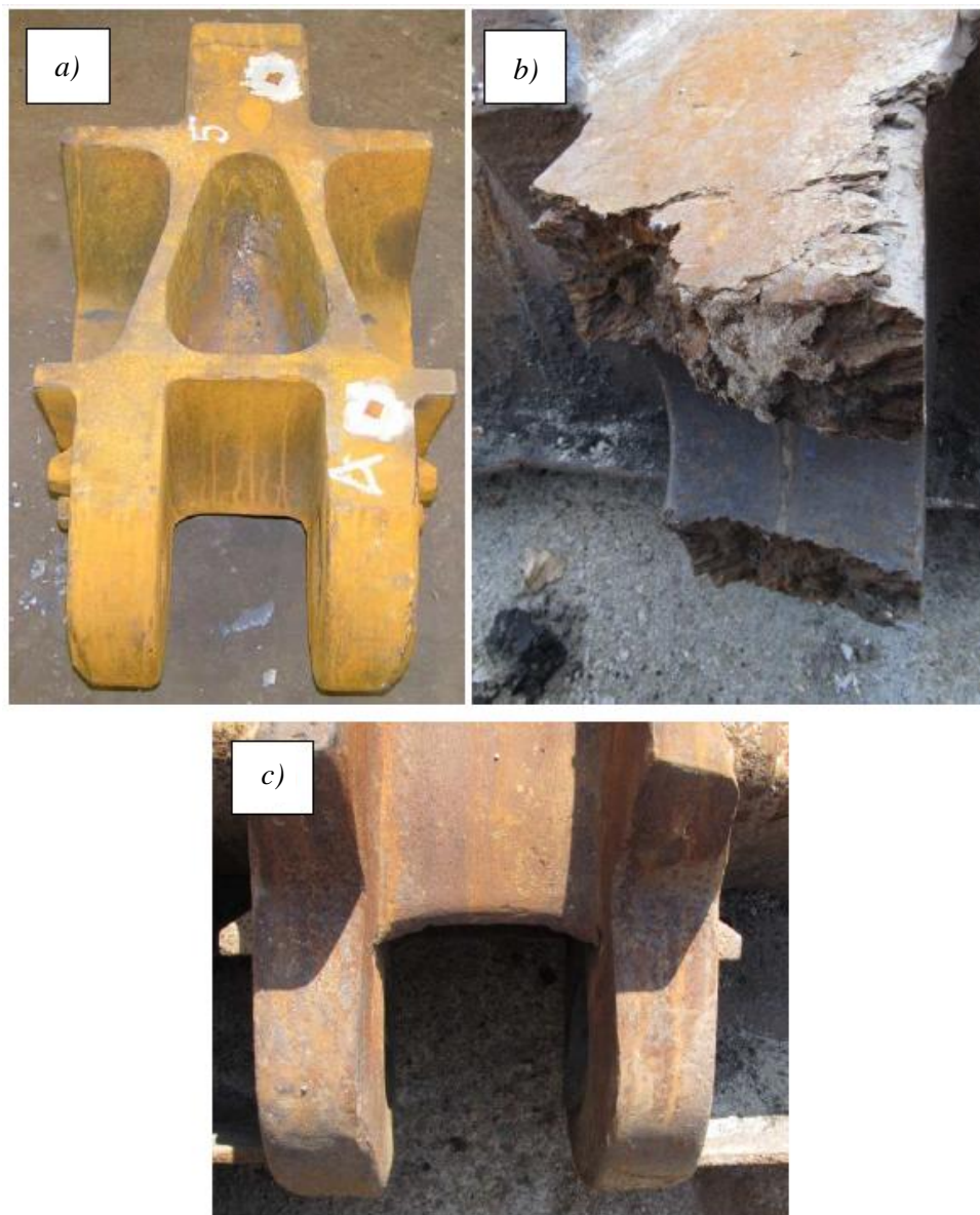
Fig. 2: Caterpillar chain links: a) Bottom view of a part in a good technical state; parts with typical failures; b) Torn-off lug; c) Plastically strained lugs. Source: author's archive.
