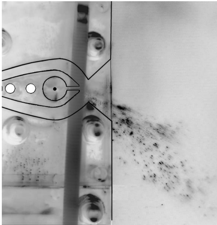
Fig. 25: Photograph (again in the inverse grayscale) of the spray generated with the water-injection body again in its place. Velocities are higher, kinetic energy is not lost inside the interaction cavity with the complex internal flow. High speed: recognisable from smearing the droplet pictures despite the very short exposure time 39 \mu s
