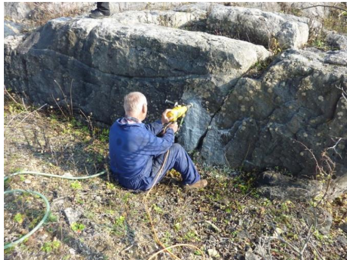
Fig. 1: Samples taking using portable core drilling machine (Holzer, 2013).
