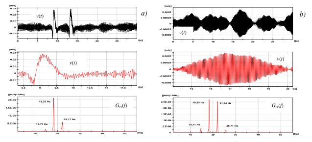
Fig. 3: Time histories v(t) and PSD  $G_{vv}(f)$  during: a) Monitoring (BK3); b)  $2^{nd}$  series of tests (BK5).
