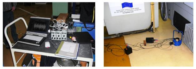
Fig. 1: Set of accelerometers with amplifiers and measuring PC in acquisition configuration to measure floor and mounts vibrations of the CNC lathe MORI SEIKI SL–204 (BK4).
