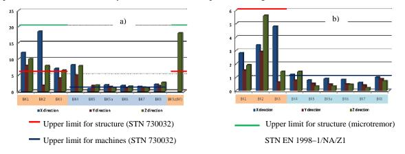
Fig. 2: Amplitude of extreme velocities values  $v_{max}$  (mm/s) of the tests: a)  $1^{th}$  series and monitoring; b)  $2^{nd}$  series.
