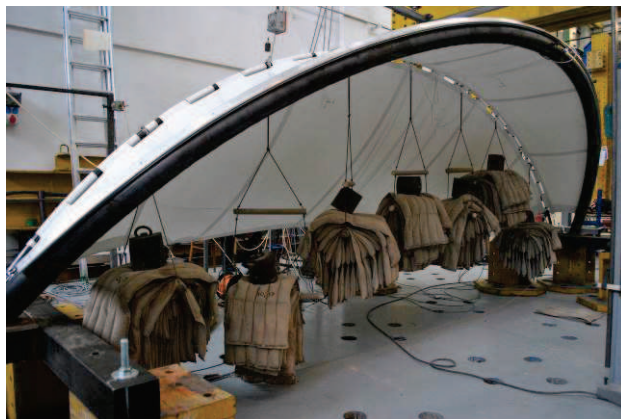
Fig. 2: Symmetrical loading of complex structure (left); Comparison of experimental horizontal deflections and numerical (SOFiSTiK) ones with various prestressing (right)
