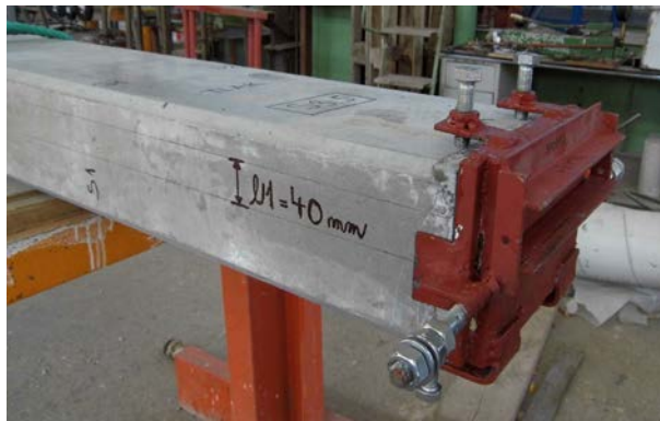
Fig. 1: Steel head for ensuring of initial eccentricity
