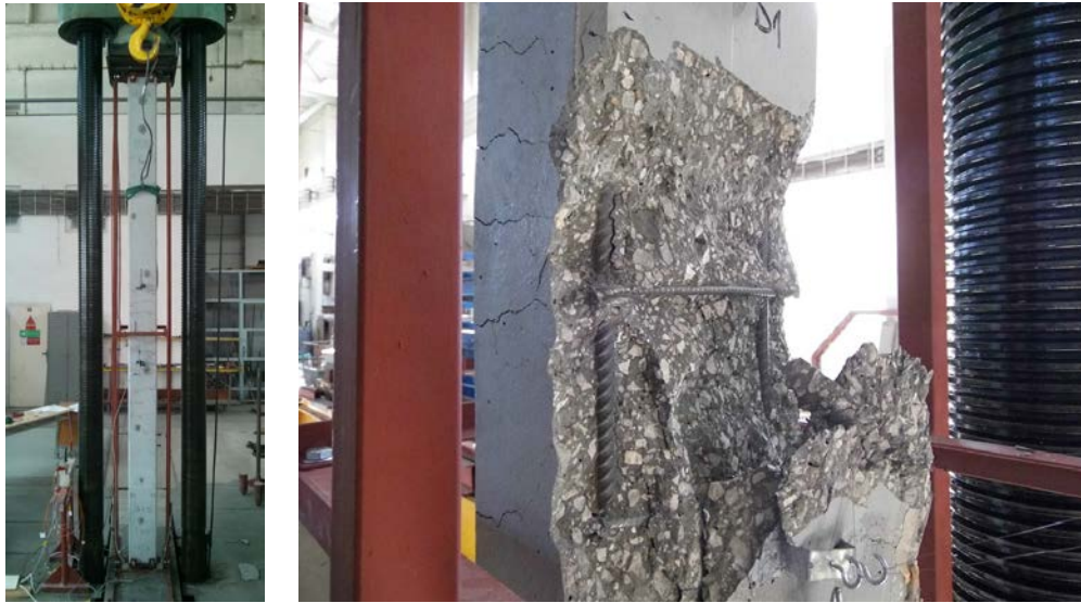
Fig. 4: Column testing (on the left), column after failure (on the right)
