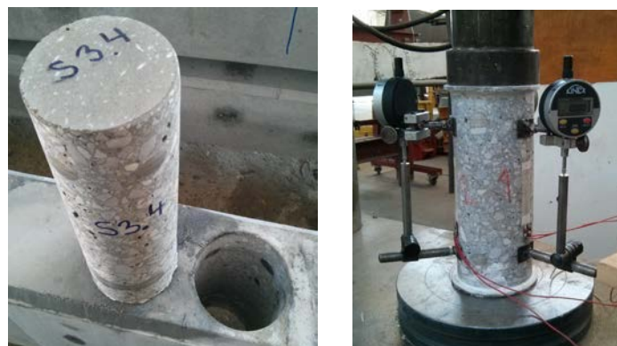
Fig. 3: The core samples for testing of concrete material characteristics
