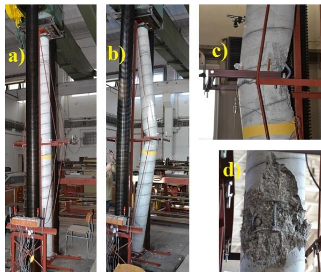
Fig. 3: a) The column before test; b) the column after failure; c, d) the detail of column failure
