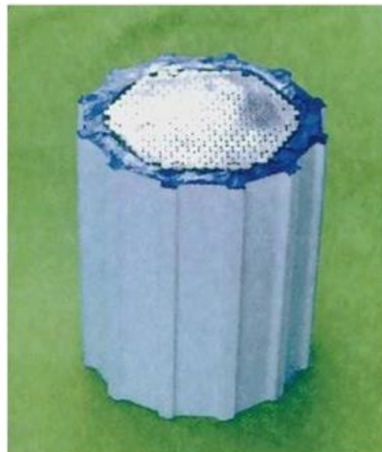
Fig. 3: Cable surface modification on the Higashi-Kobe bridge.
