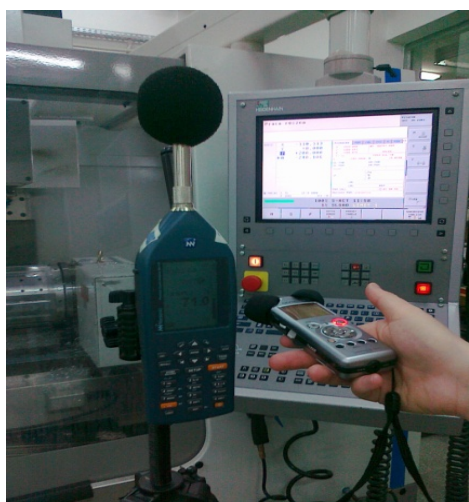
Fig. 1: Measurement position in the operator's work zone of CNC milling machine (Błasiak, M. et al., 2015).
