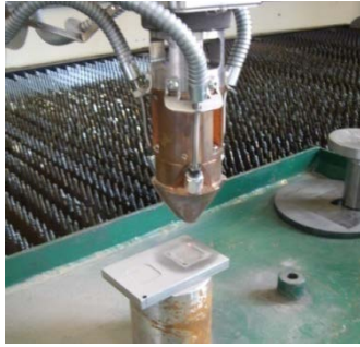
Fig. 2. Head used for cladding and the process of cladding (Wijas & Nowakowski, 2015)
