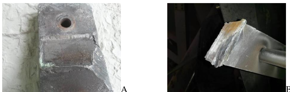
Fig. 5. Sheared welded joint between the hammer (A) and the mount (B).
