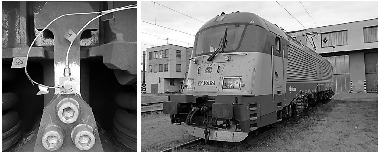
Fig. 1: Acceleration sensor placing on the wheelset axle box of measuring vehicle (illustration photo).
