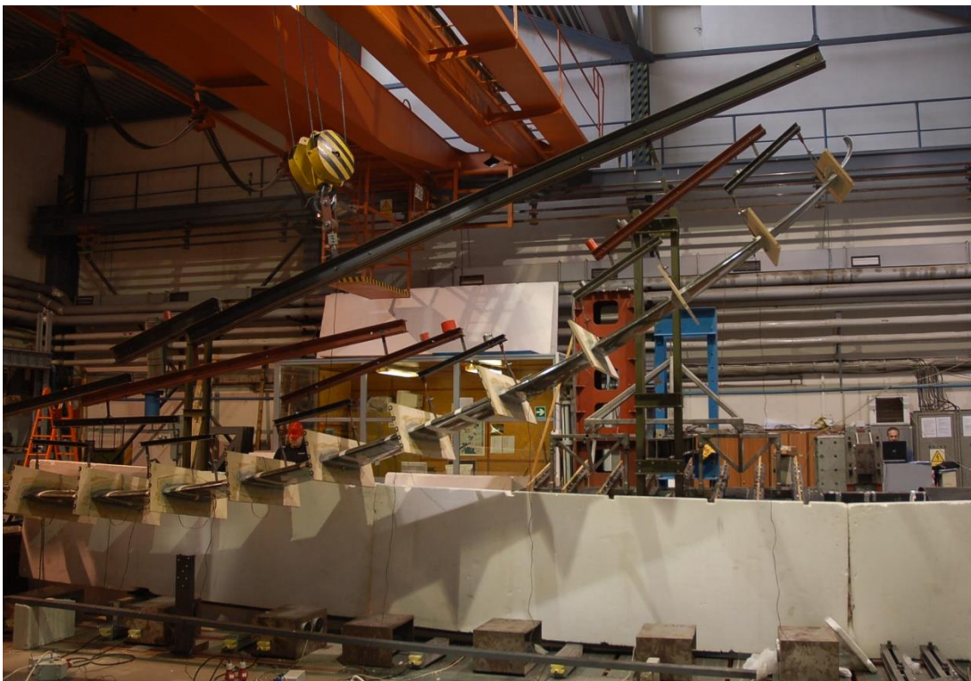
Fig. 1: Composite wing structure test.
